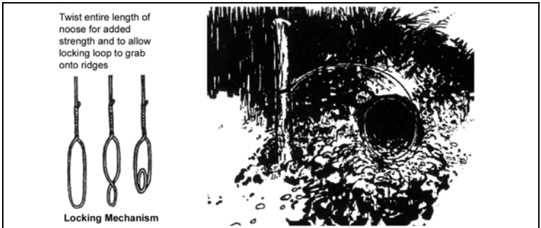
Figure 11-8. FORMING A LOCKING-TYPE SNARE LOOP
